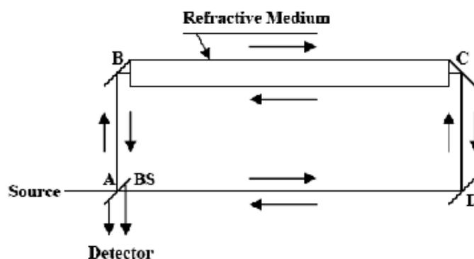
**Fig. 1** Hoek's experiment: Light from the source is split into two beams by the beam splitter BS. One of the beams follows the path ABCDA, and the other ADCBA. The beams are recombined in A to form an interference pattern in the detector. The segment BC is occupied by a refractive medium, while the other parts of the circuit consist of air at atmospheric pressure
