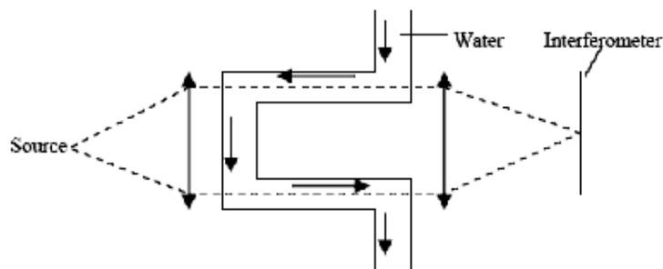
**Fig. 2** Fizeau's experiment: Light from a source is split into two beams, which are sent toward the two branches of a pipe filled with water before being recombined to form an interference pattern. When the water starts to flow, the fringes are shifted. The fringe shift permits to deduce the variation of the speed of light due to the flow.
